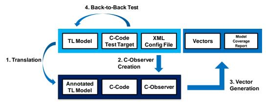
Figure 4: Simplified Workflow within BTC EmbeddedTester
