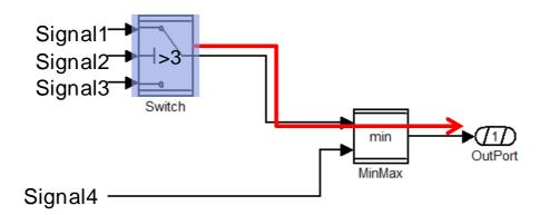
Figure 2: Observability Path from Switch Block to visible OutPort
