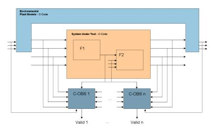
[BTCEW2010]. The assumptions of the contracts will be used to automatically synthesize the Environmental part of the verification/test architecture which is visualized in the figure above.
