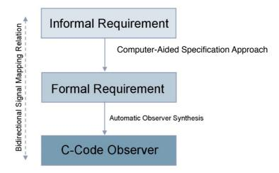
The presented technology<sup>1</sup> shall address this challenge by introducing a computer-aided process accompanied requirement specification method, which can be used from the very beginning of the development process. It starts with text written in natural language and it ends up with a machine readable C-Code-Observer description, which is used for automatic test and verification purposes.
